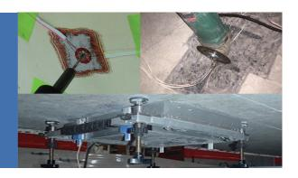
At Josei, we conduct residual stress verification on steel and concrete structures using measurement techniques based on the principle of stress relaxation to verify the safety performance of structures affected by forced deformation.
