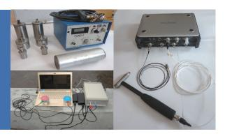
Non-destructive testing using elastic waves primarily includes ultrasonic methods, impact elastic wave methods, and AE methods. These techniques are classified based on differences in how elastic waves are transmitted and received, as well as the frequency range in which they propagate. At Kamiharu, we perform various non-destructive tests using elastic waves to meet the specific objectives of each investigation.
