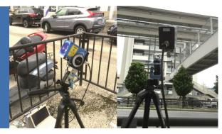
Actual stiffness of bridge girders and similar beam structures: To evaluate EI, methods such as ① calculating natural periods from vibration measurements or ② measuring displacements generated during loading tests are implemented. At Kamiharu, we simultaneously measure both items (① and ②) using a medium-range laser Doppler measurement device, without causing local community impacts such as traffic restrictions or work stoppages.
